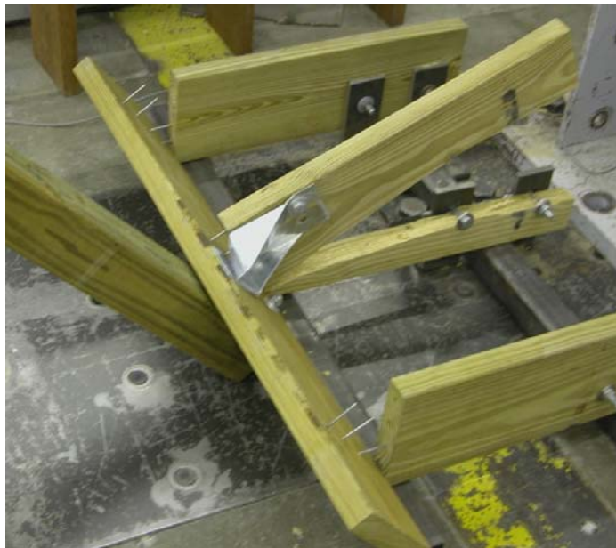
Figure A6. Failure mode for test specimen 1, configuration 3
