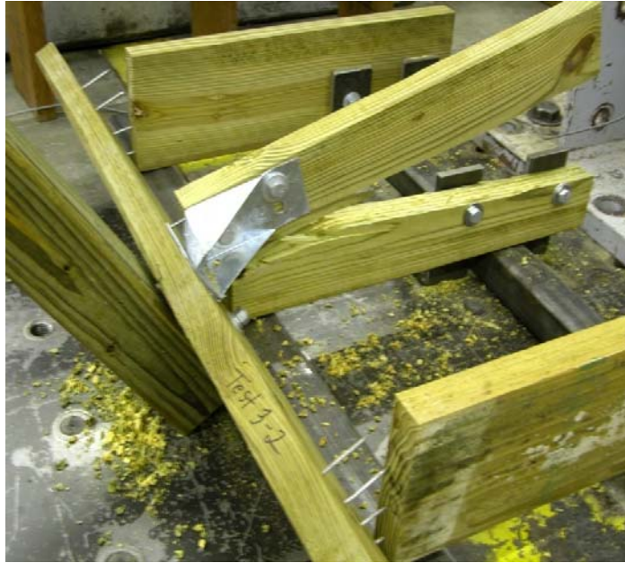
Figure A7. Failure mode for test specimen 2, configuration 3
