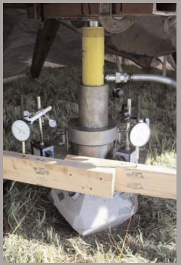
Bearing Load Test - Pier and Pins Push against the Soil as a Single Solid Shape.
